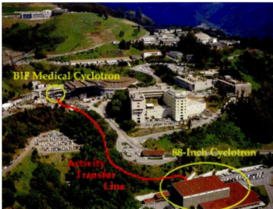
The BEARS project has delivered its first radioactive beam. It includes a specially built 300 m long, 15 cm diameter transfer line.
